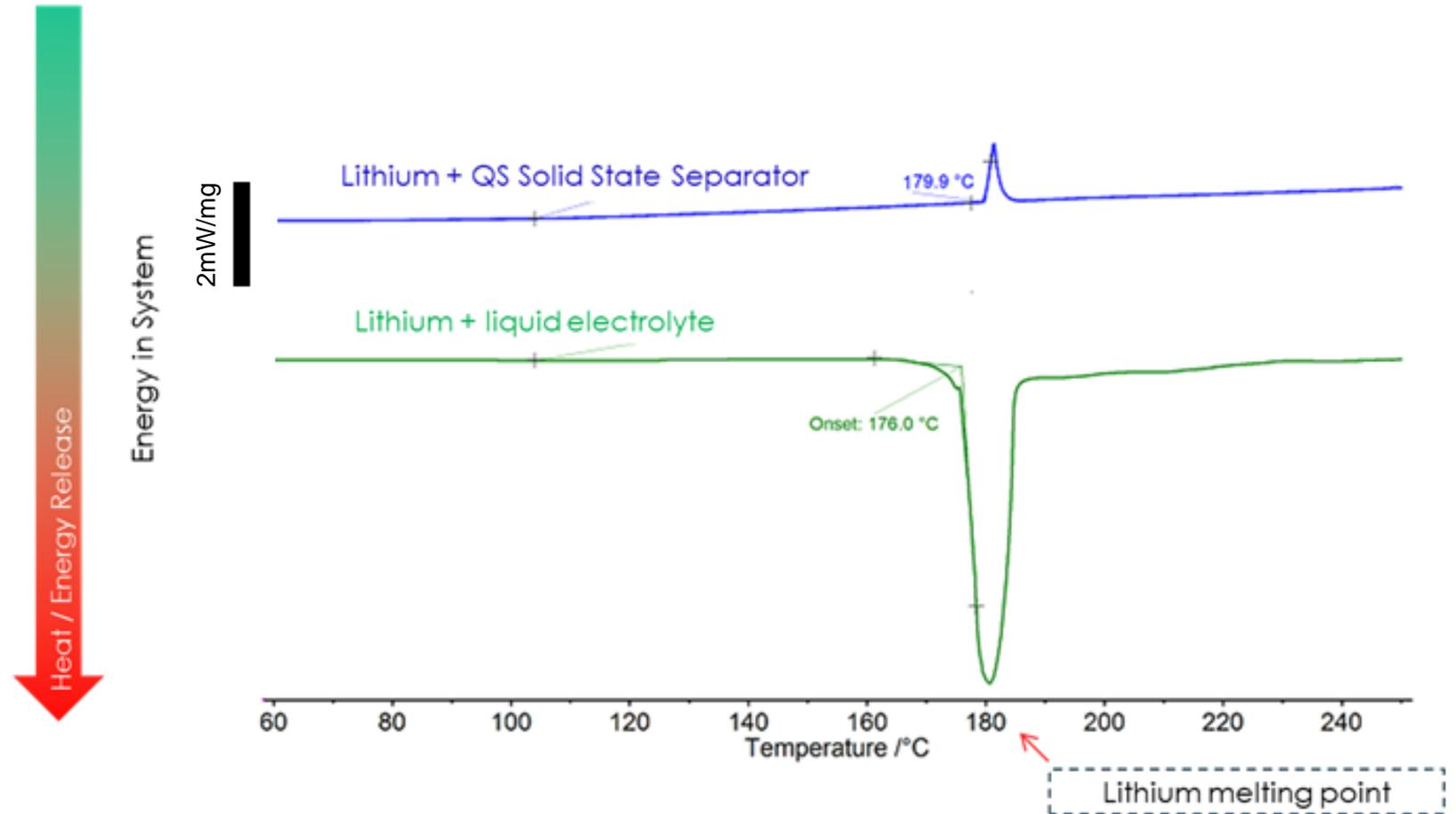
Unlike a liquid electrolyte, QS solid-state separator has no appreciable reaction with molten lithium metal
